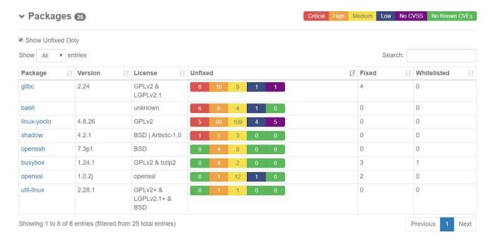
Vigiles is optimized for embedded systems and filters vulnerabilities based on a project's Linux kernel configuration and U-Boot configuration, which removes vulnerabilities affecting features not being used. This reduces vulnerability investigation and triage tasks by 75 percent on average.
