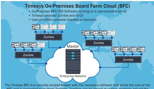
The Timesys BFC is a centrally located Master with the necessary software that forms the core of the BFC and is connected to multiple Zombies. Zombies can be placed at various locations around the corporation, as long as the Zombie has network connectivity to the Master.
